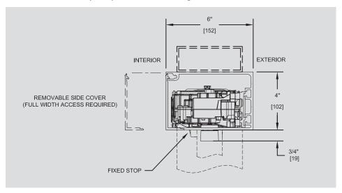
Elevation view Overhead concealed operator center hung Right hand door shown (left hand opposite)
