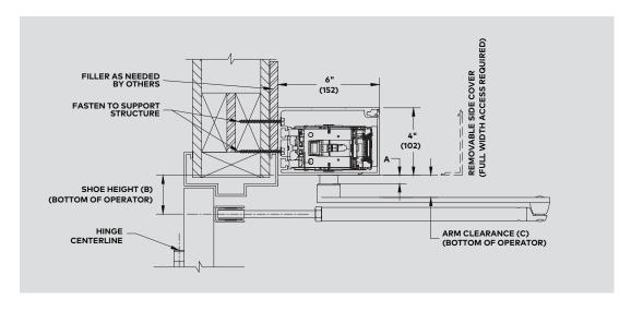
Elevation view 4x6 Narrow Header single push operator Left hand door shown (right hand opposite)
