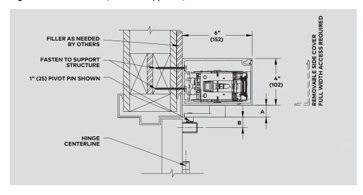
Elevation view 4x6 Narrow Header single pull operator Right hand door shown (left hand opposite)
