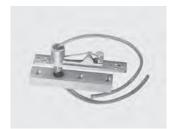
E80622, 2 wire/E80624, 4 wire— Electrified walking beam top pivot for power transfer. Available in a two-wire and four-wire design using #18 AWG. Both designs provide a maximum of 6 A @ 24 V. Specify number of wires required
