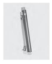
**ES105**—Power transfer with steel housing and flexible tube. Secure and inconspicuous channel to bring power from frame to door. Narrow, shallow channel easily mortises into door edge. Accepts up to 5/16" dia. wire bundle. Accommodates doors that swing open 120°. Concealed when door is closed. Suitable for wood, aluminum, or steel applications.
