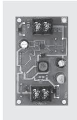
**24-12CONV**—Converts 24 VDC current input to 12 VDC output 1.5 A output @ 12 VDC.
