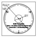
Figure 2-2 The Drill Template
