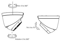
Figure 2-35 Adjust the Lens
