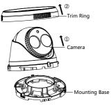
Figure 2-9 Disassemble the Camera
