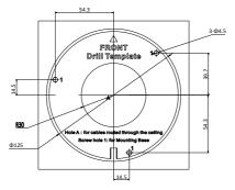
Figure 2-32 The Drill Template
