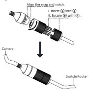
Figure 2-44 Waterproof Accessory Installation
