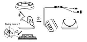
Figure 2-23 Disassemble the Camera
